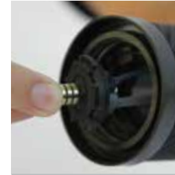
Insert the Coaxial Plug and Lock Ring on the Lamination Collar.
