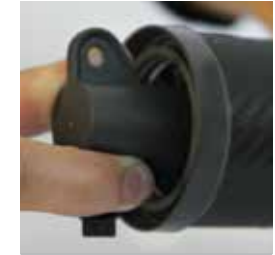
Use the Coaxial Installation Tool to secure the assembly.
