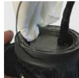
Cleaning the Lamination Ring.
