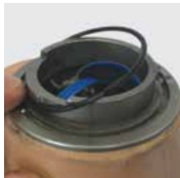
Installing lubricated O-ring.
